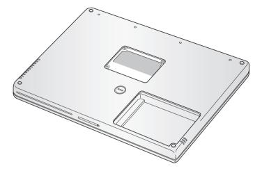
7 Replace the memory door and screw it into place.
